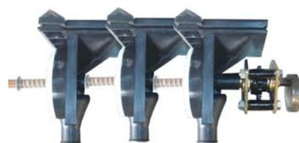
*Thian seed modules. Note drive unit for agitators on right hand end of string of modules Plate 1. Applied use of Thian seed module with excellent cross over of technology to small-scale continuous seeders for mechanization of field experiments and other small-scale agriculture, horticulture, viticulture, wildlife management and recreation.*
