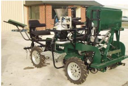
*S&N Flexiseeder plot drill (delivered to Norway) fitted with Thian fertilizer box.*
