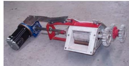
*Digi-gearbox retro-fitted to Accord Cell wheel as test bed.*
