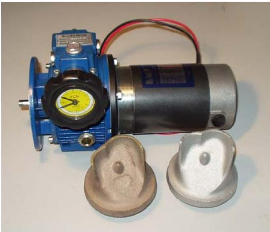
Left: Flexiseeder Brooks-S&N mechanical variator including two impellor blocks, one cast in bronze and the other aluminium.
